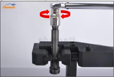
A The tightening torque of the nozzle cap must be installed in accordance with the tightening torque specified in the injector maintenance manual.
