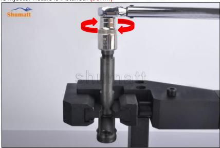
$lack lack \Delta$  The tightening torque of the nozzle cap must be installed in accordance with the tightening torque specified in the injector maintenance manual.
