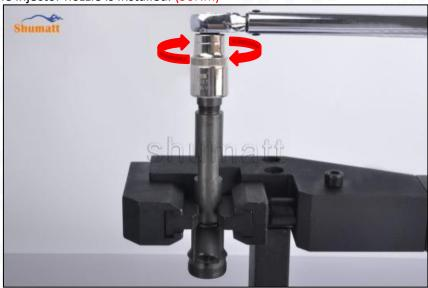
lacktriangle The tightening torque of the nozzle cap must be installed in accordance with the tightening torque specified in the injector maintenance manual.
