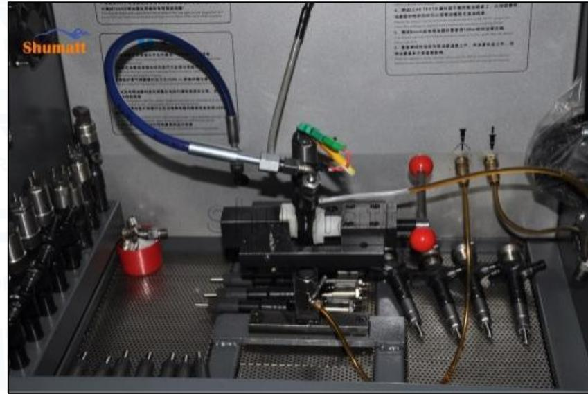
**⚠** The correct injector type should be selected for testing
